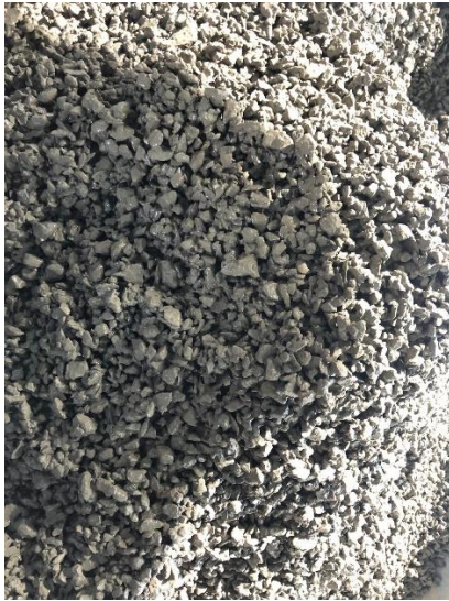
Concreto permeable fresco
