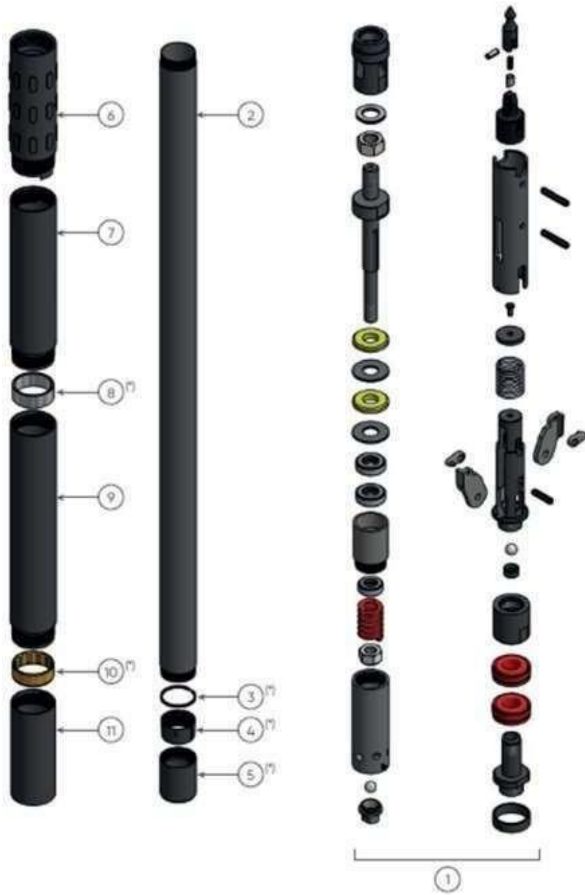
Figura 9. HO-LINK LATCH HEAD ASSEMBLY MK II-100400300201
