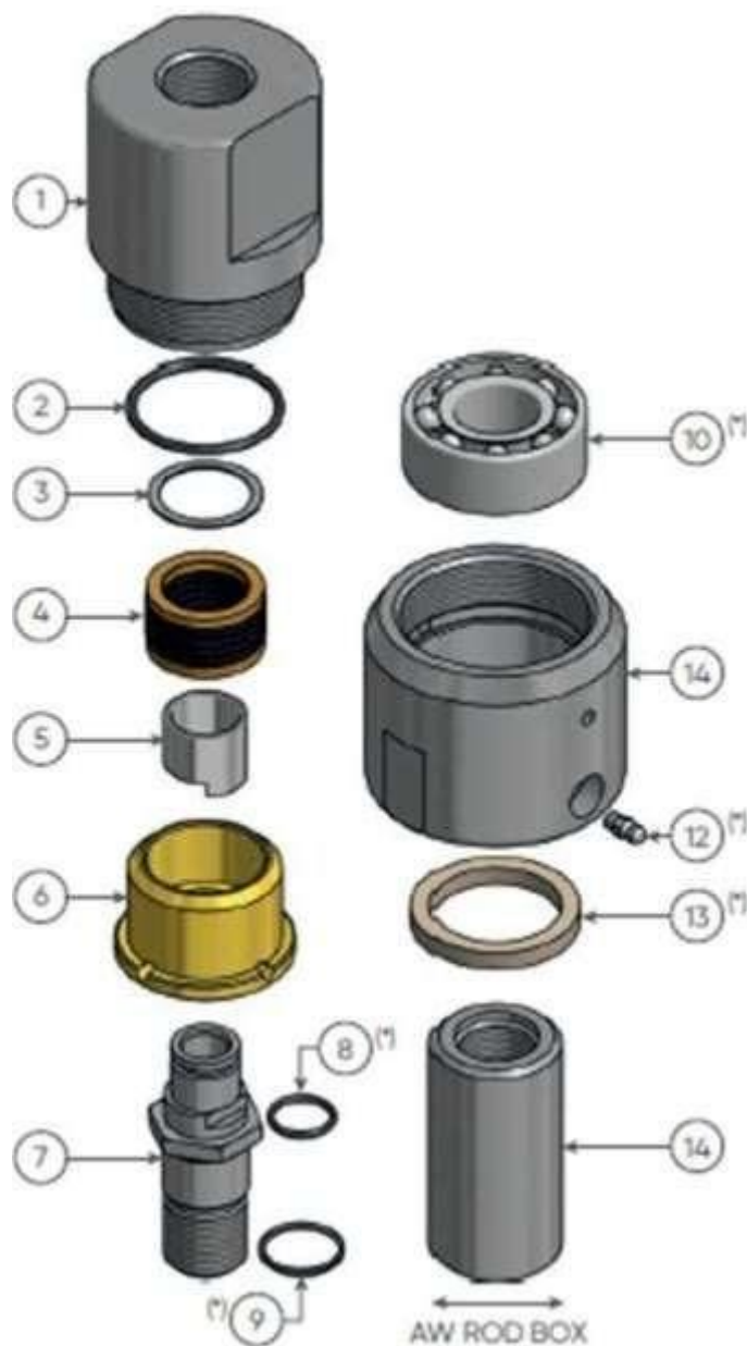
Figura 11. 5K UNDERGROUND COMPACT WATER SWIVEL ASSEMBLY (AW ROD BOX) -245200100105
