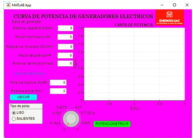
Figure 7: Completed graphical interface for both smooth pole generators and protruding poles.3
