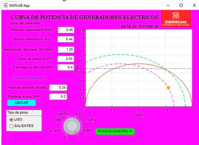
Figure 10: The operability region of the synchronous generator is defined by the excitation field current, which avoids over-generation.
