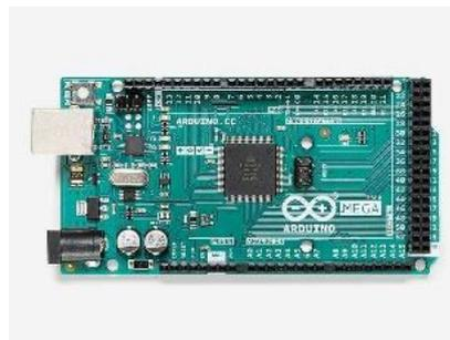
**Figura 6. Arduino Mega**
