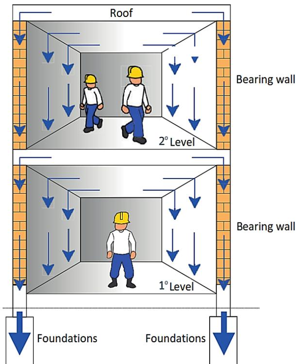
Figure 8. Load distribution of load-bearing wall [27]
