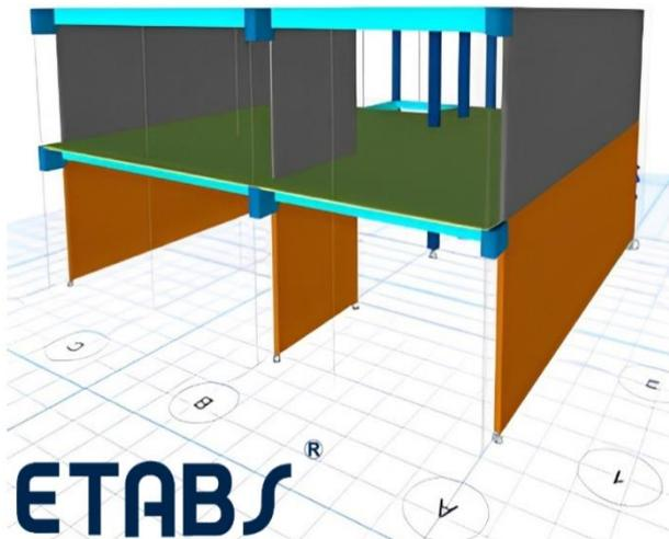
**Figure 9.** Structural analysis in frame structures with infill masonry walls houses
