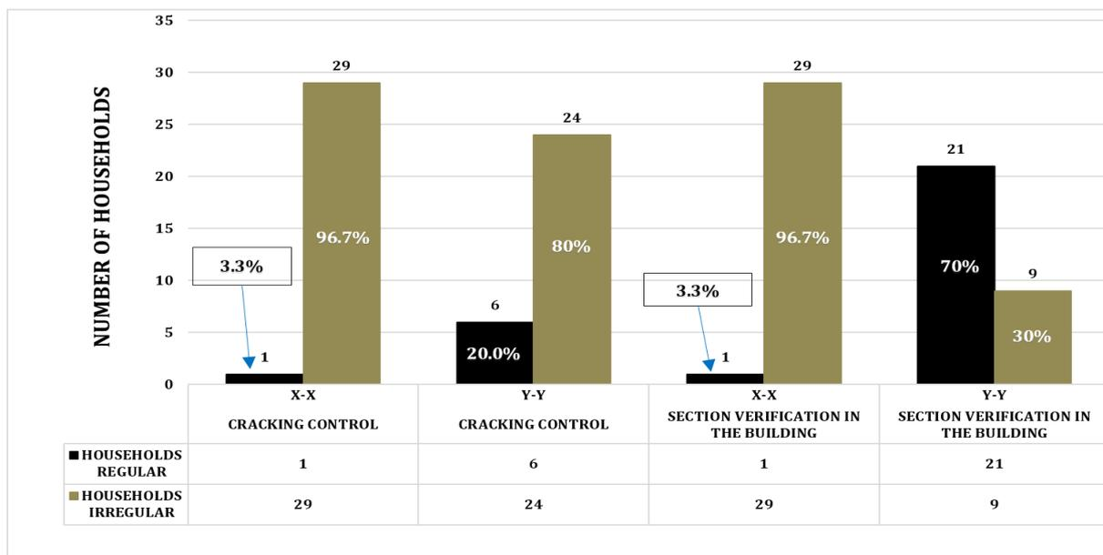
Figure 16. Crack control and shear verification
