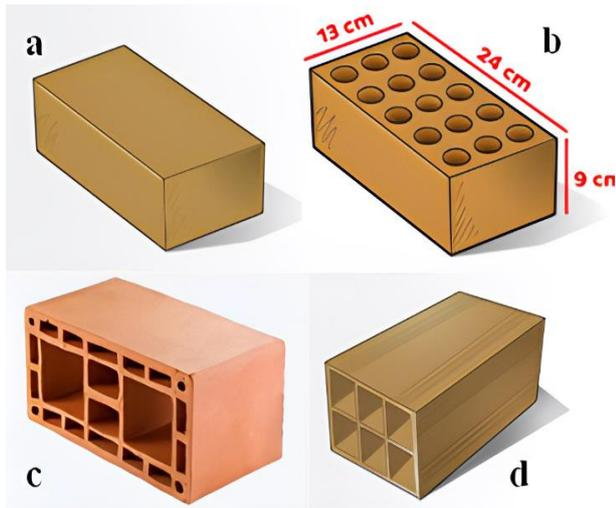
Figure 7. Types of bricks: a) Solid brick, b) Hollow brick, c) Hollow bricks, d) Tubular bricks
