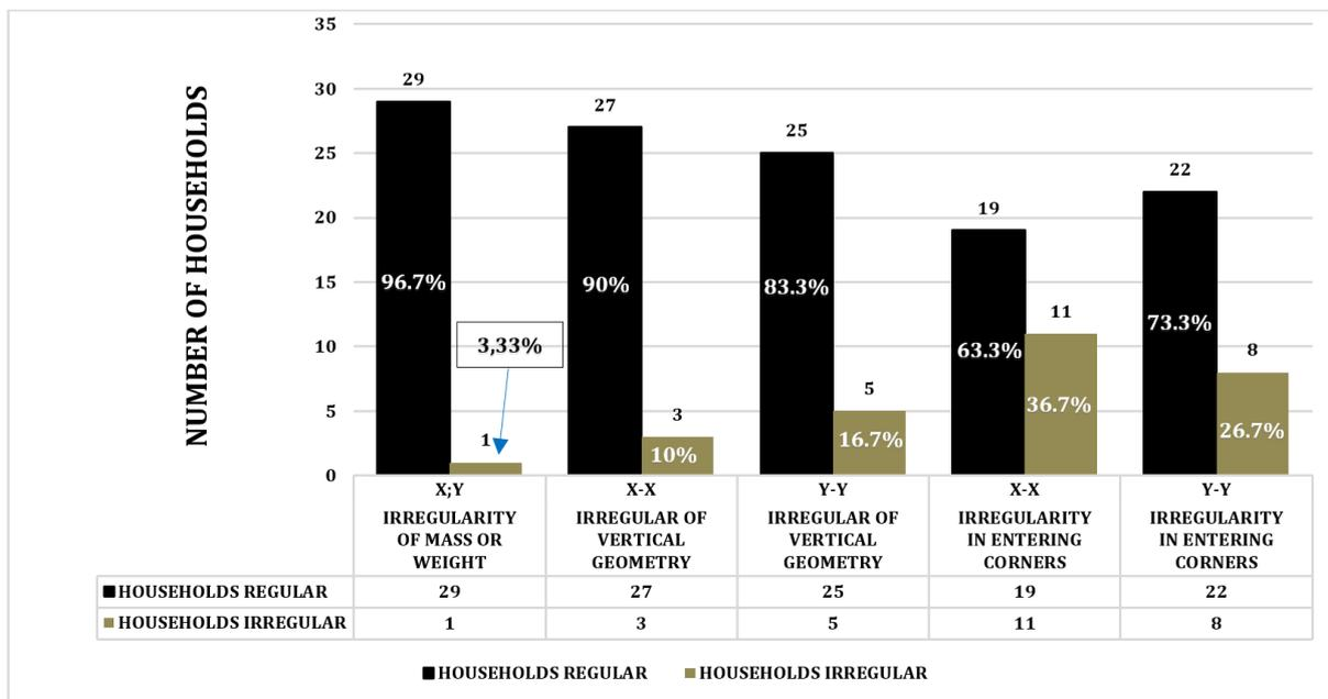
Figure 14. Irregularities in floor plan, height, and mass in frame structures with infill masonry walls house
