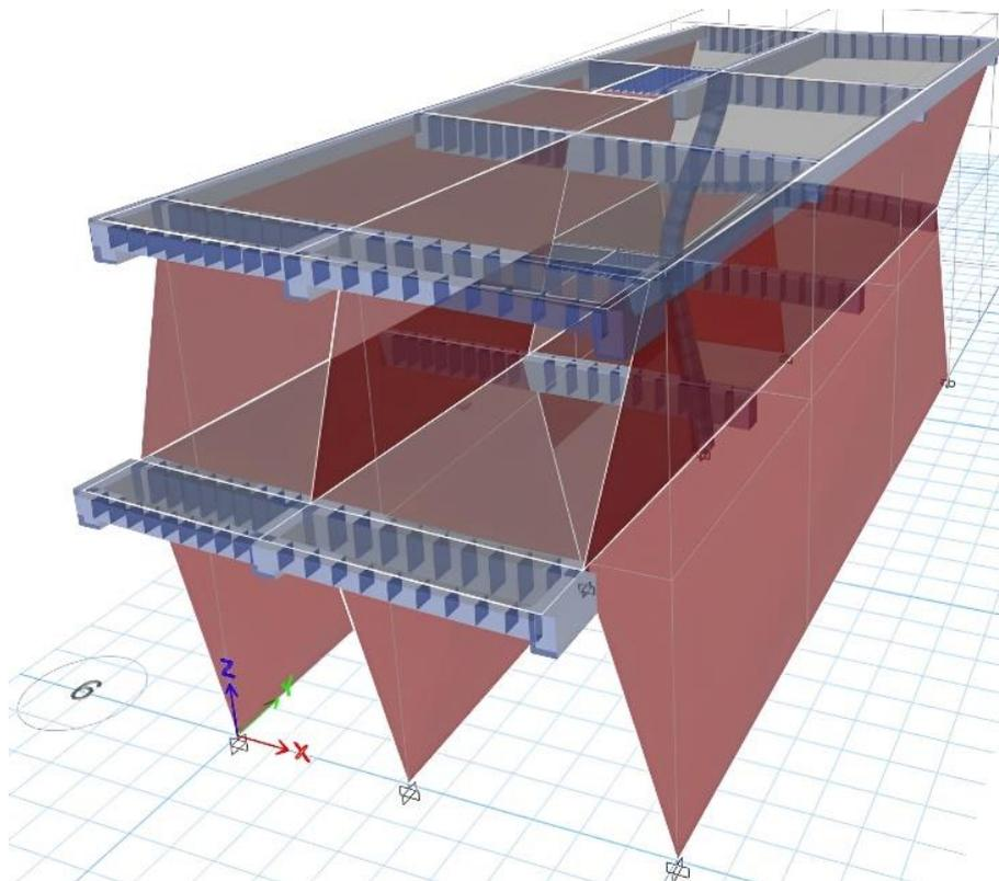
Figure 18. 3D view of the analysis of House 8 – ETABS
