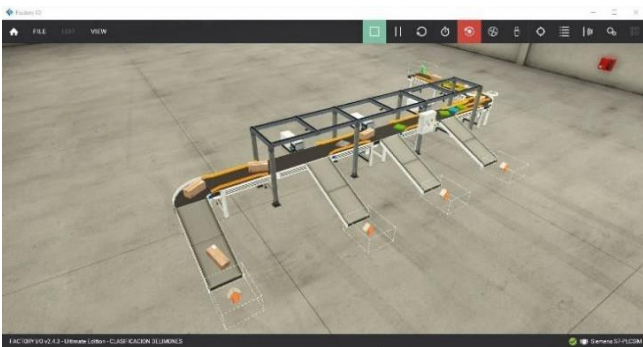
Fig. 11. Detection of brown boxes (rotten lemon).
