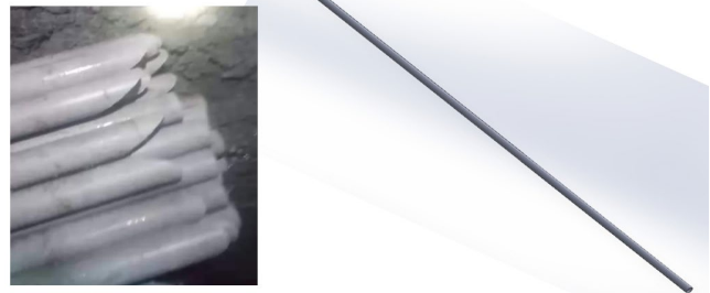
Fig. 3. Charging tubes for loading explosives
