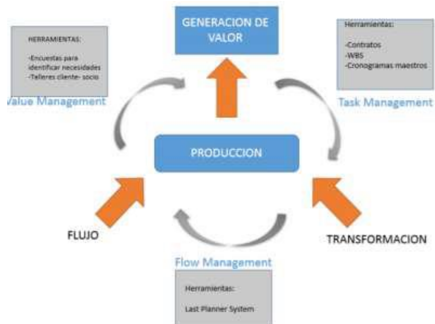
Figura 15. Herramientas de Lean Construction
