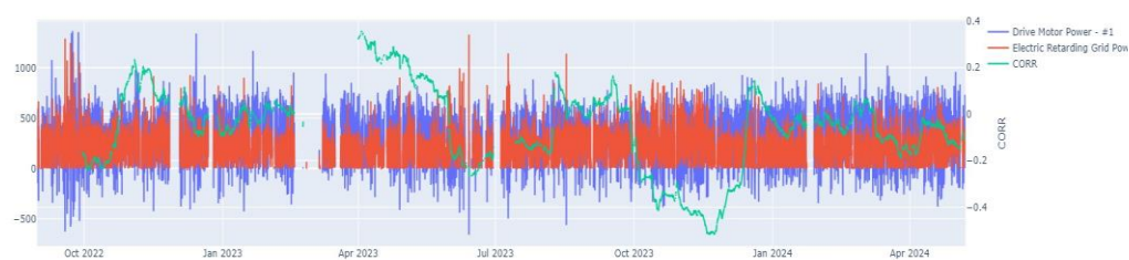
CM503 - Drive Motor Power - #1 vs Electric Retarding Grid Power Consumption - #1
