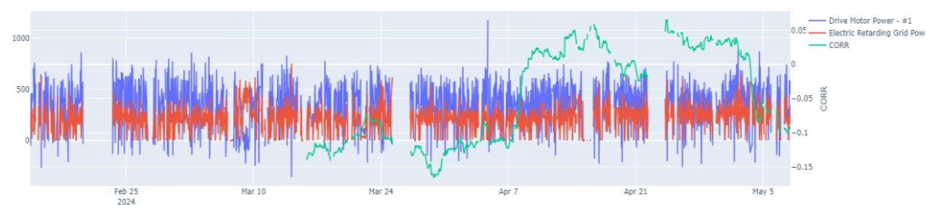
CM507 - Drive Motor Power - #1 vs Electric Retarding Grid Power Consumption - #1
