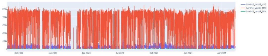
CM503 - Electric Retarding Grid Power Consumption [kW]
