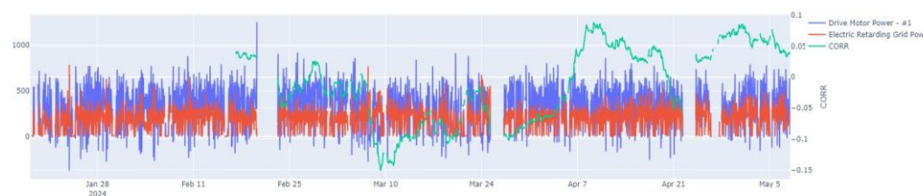
CM505 - Drive Motor Power - #1 vs Electric Retarding Grid Power Consumption - #1
