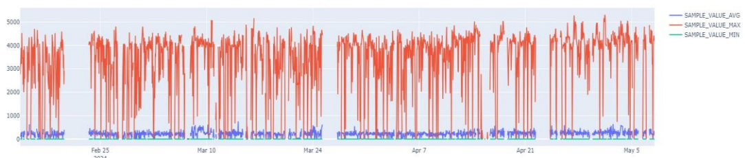
CM507 - Electric Retarding Grid Power Consumption [kW]
