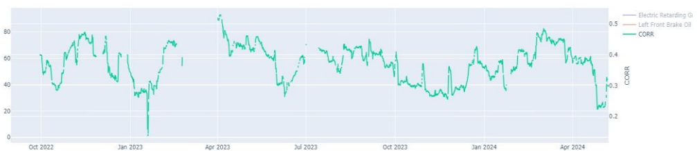
CM503 - Electric Retarding Grid Power Consumption vs Left Front Brake Oil Temperature
