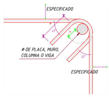
DETALLE PARA EL DOBLADO DE ESTRIBOS EN COLUMNAS SIN ESCALA
