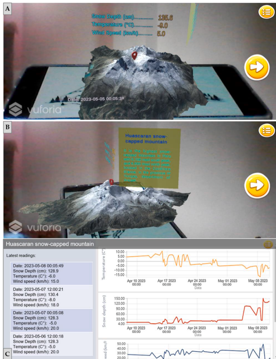
Fig. 13. IoT and AR application showing in: A. They show the data captured by the sensor: depth, temperature, wind speed, date of reading the data and location belonging to the first scene; B. Description of the snow-capped Huascarán. C. History and graphs of the behavior of the data belonging to the second scene.
