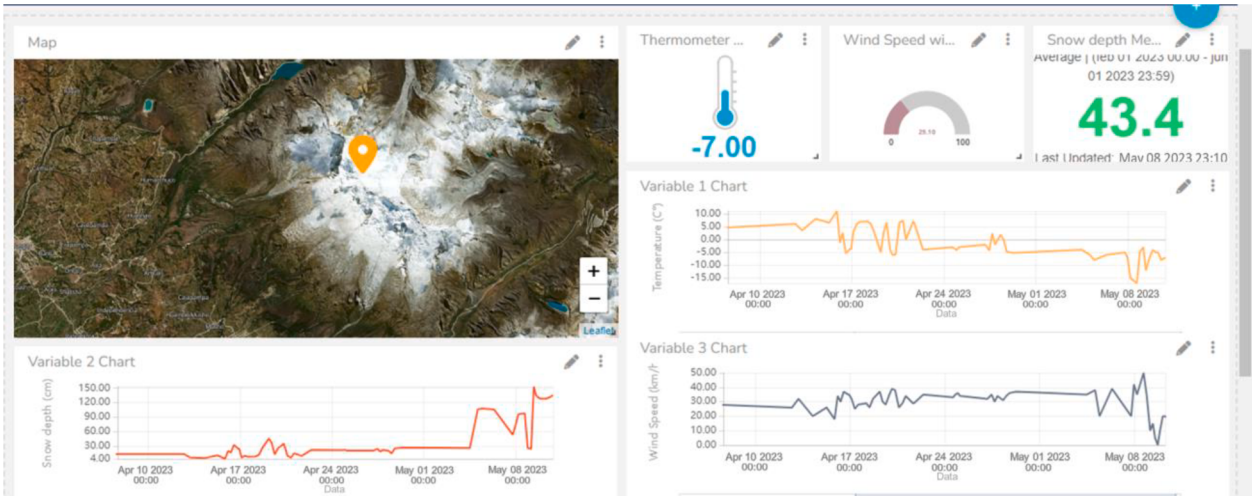
Fig. 9. Dashboard view of variables in Ubidots for real-time data visualization.
